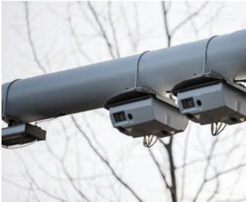
Image 3: Example of the redundant VDX2i sensor positioning at the portals
