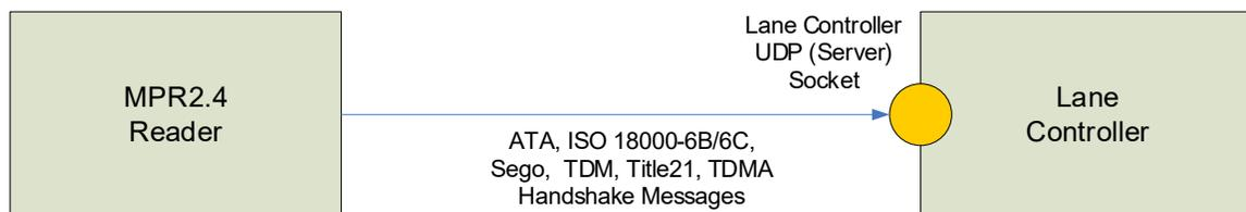
**Figure 2.13-1: JANUS MPR2.4 Reader / Lane Controller Handshake Messaging (UDP) Sockets**
