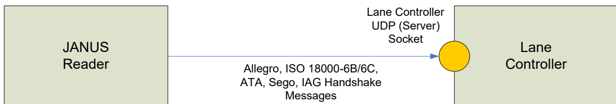
Figure 2.12-1: JANUS MPR2.3 Reader / Lane Controller Handshake Messaging (UDP) Sockets
